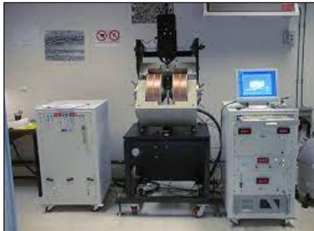
Figure (3.11): Vibrating sample magnetometer (VSM) instrument.
