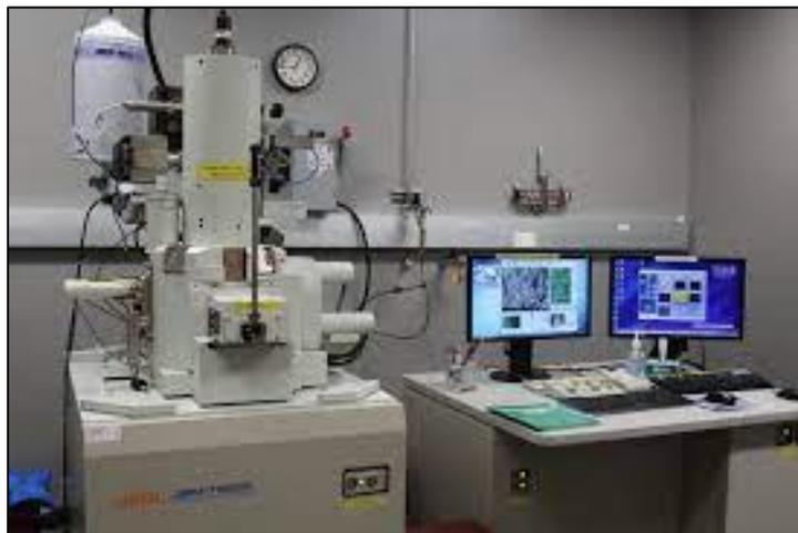
**Figure (3.10): Photograph of field emission scanning electron microscopy instrument.**
